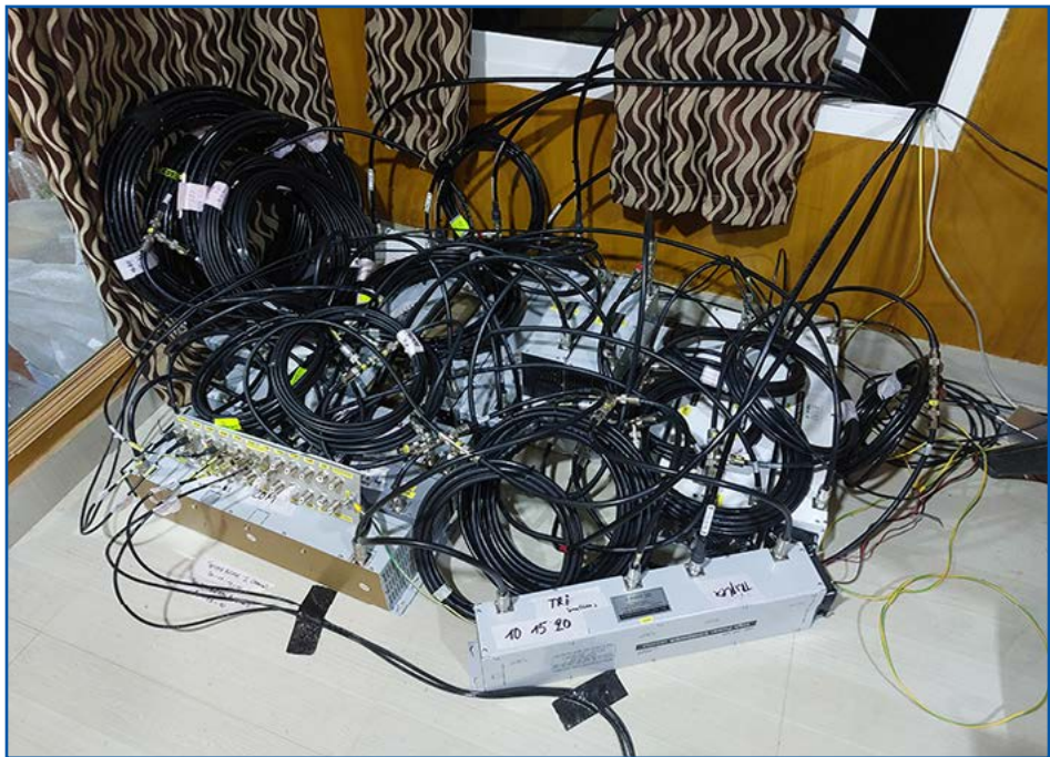
This jumbled mess was our functional patch panel, filters, stubs and stops.
