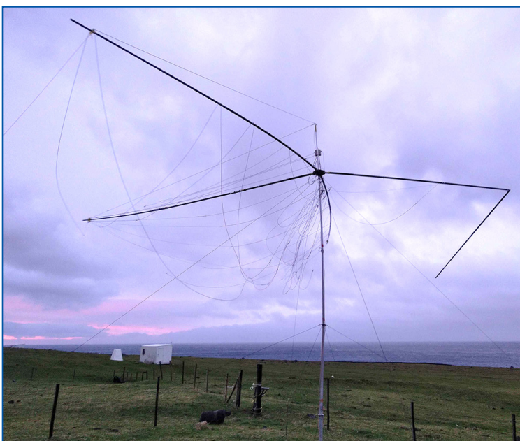
The result of antennas battling high winds: Spiderbeam (left) and LBS vertical.
