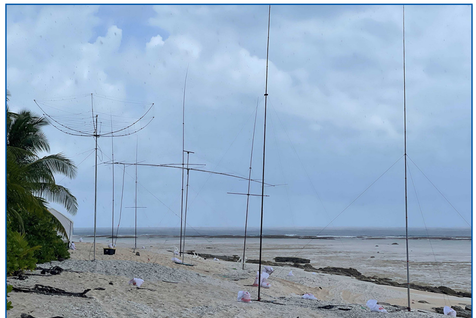
VDAs, Hexbeam and 8-element 6M beam antennas on the beach.
